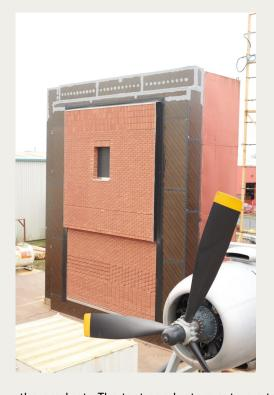
Air Leakage - The air-tightness test assesses the performance of windows, doors, cladding, and curtain walling in resisting air penetration despite the wind loads on the products. We tested to a  $2.4 \text{kN/m}^2$  serviceability load, and a  $3.6 \text{kN/m}^2$  ultimate load., and achieved passes.
